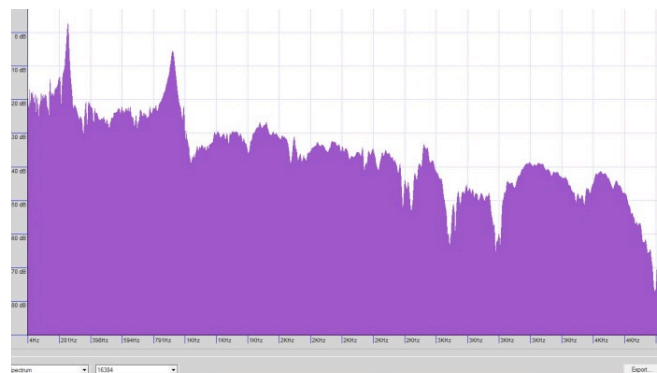
Figure 6: Audacity spectrum showing two resonance peaks.
