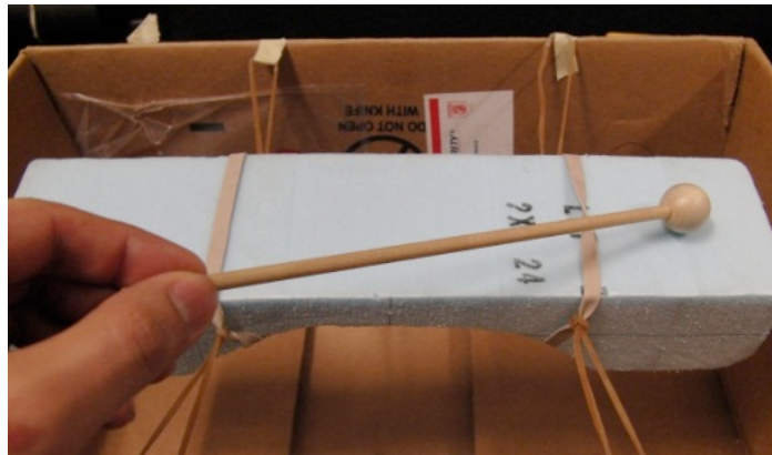
Figure 4: Styrofoam xylophone bar, suspended by rubber bands near the zero-crossings of the first resonance in a cardboard sound-box, and being struck near one end.
