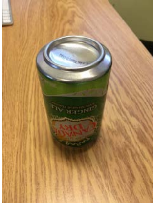
Figure 1: The bowl-shaped bottom of an inverted 355 ml Canada Dry ginger ale pop-can.
